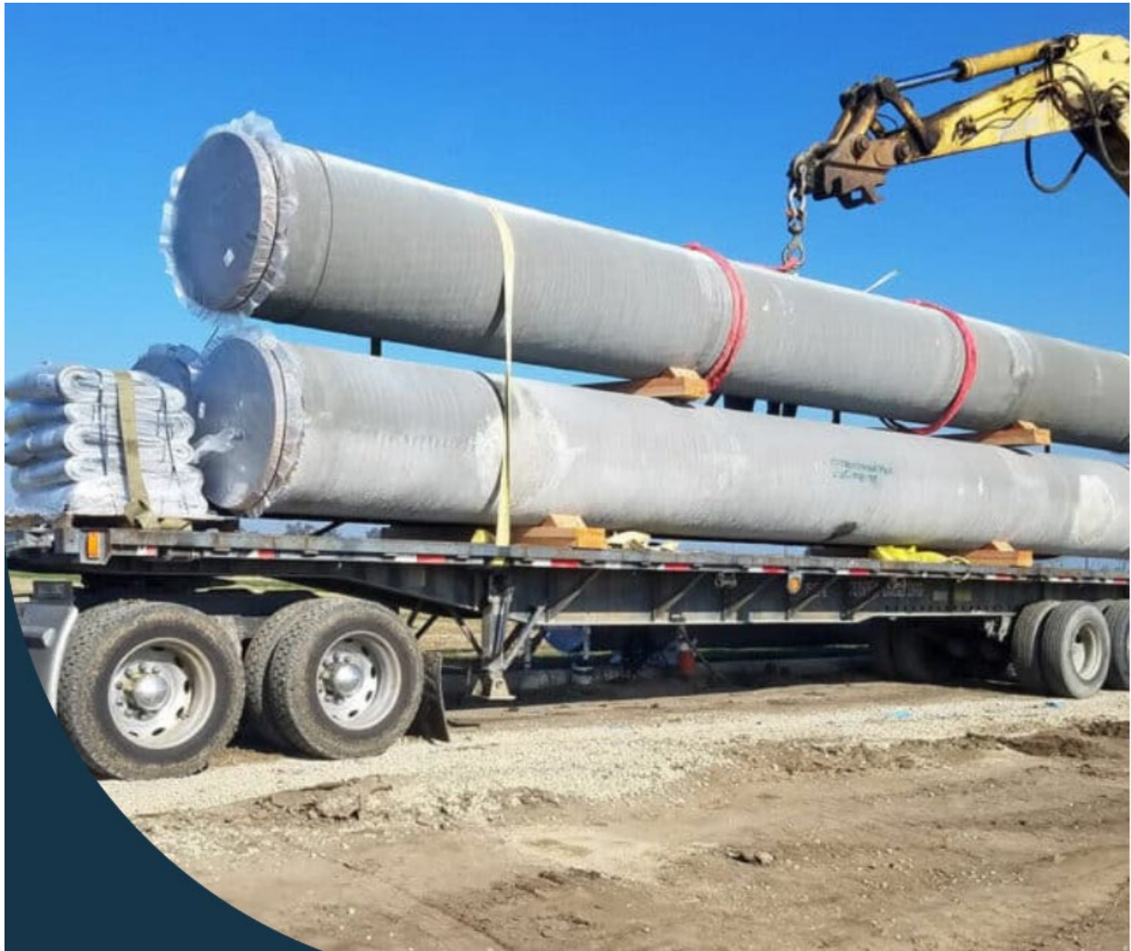
Typical WSP – Mortar Coated and Mortar Lined
