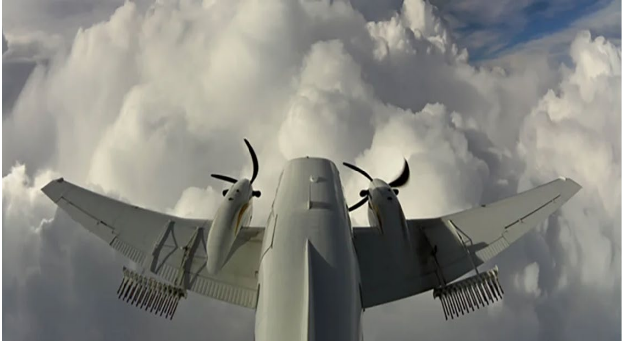
Aircraft Flying into Clouds Carrying Flares Filled with Silver Iodide for Introduction into Clouds
