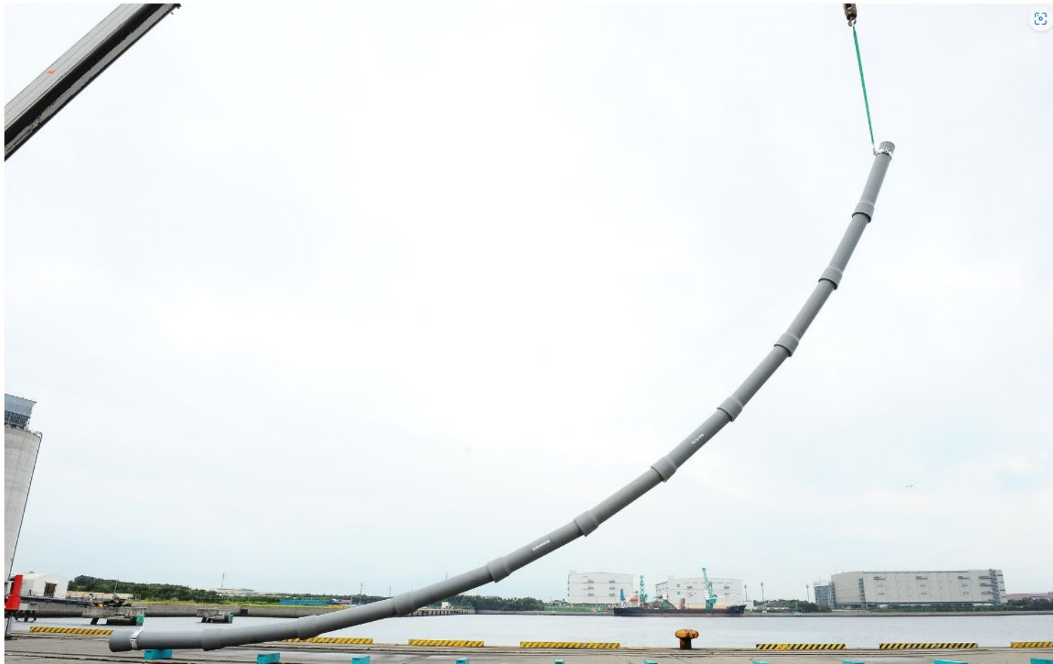
Demonstration of Earthquake Resistant Ductile Iron Pile (ERDIP) Hoisted with Crane (Kubota)
