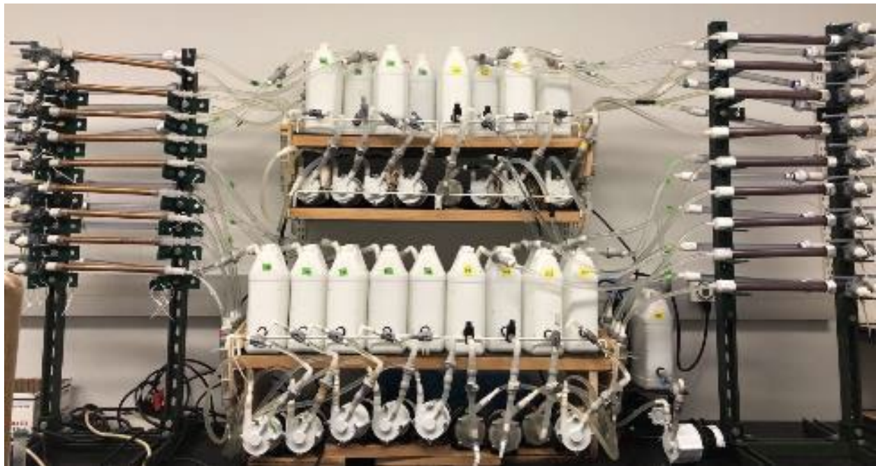
Copper Pipe with Lead Solder Pipe Loops and Brass in Pipe Loops
