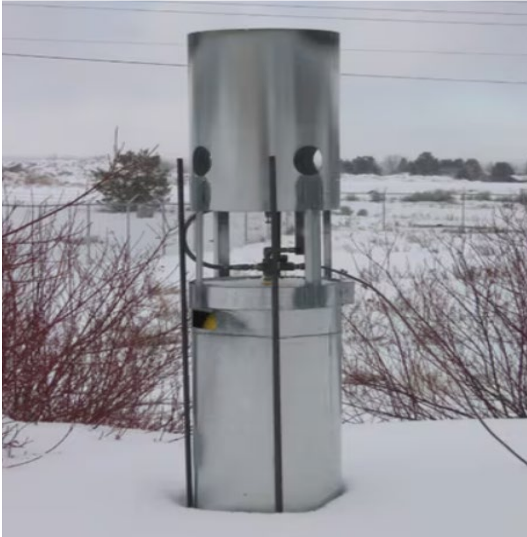
Typical Cloud Seeding Propane Generator that is used to Introduce Silver Iodide Particles into Approaching Storms to Increase Snowfall at High Altitudes
